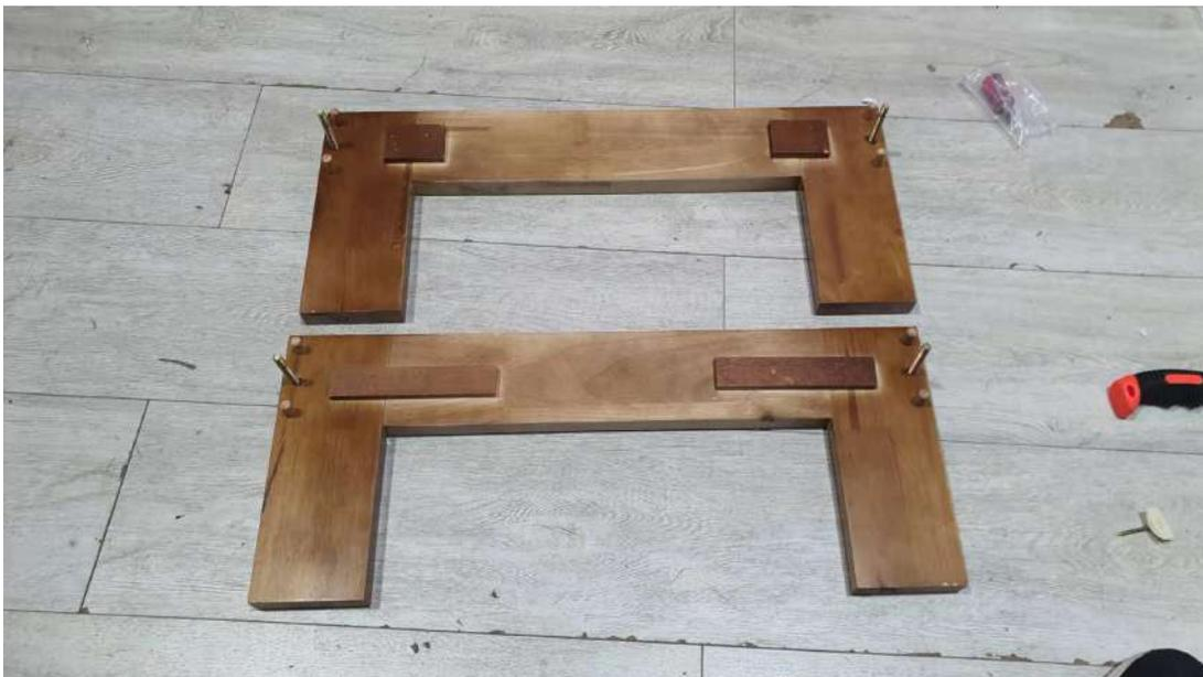
Put the wooden bars 2 each on one side and in total 8 wooden bars will be used , and put the long thread screws x 4.
