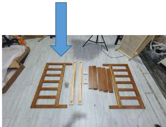
Attach the back part with the side arms with the screw shown in the pic and nut on the bottom Thread bolt .
