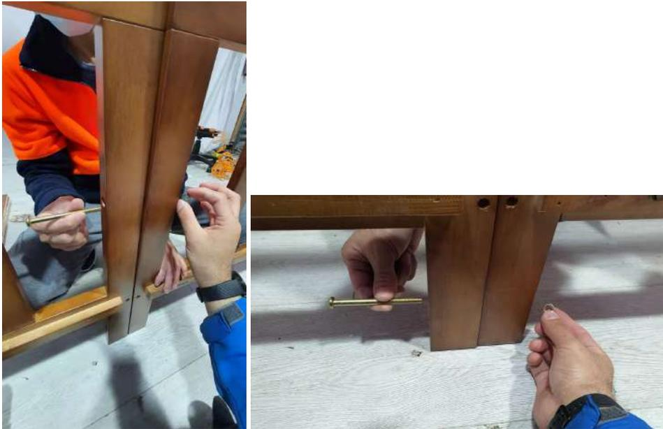
Then Join the 2 back side together with long bolt and screw as shown in the pic
