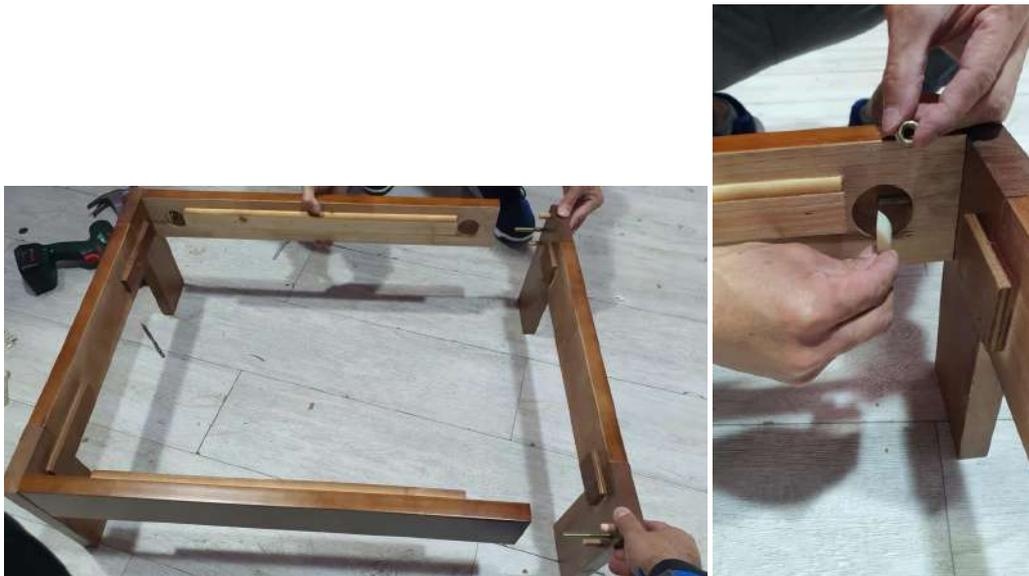
Attach the side frame with the bar and the tight with plastic round shape cover and then bolt .
