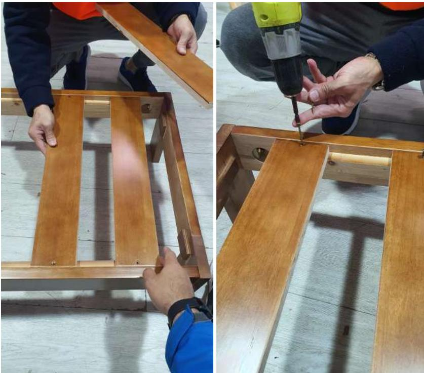
Drill the screws on the frame slats to make the base. Try to leave equal amount of space between each part.
