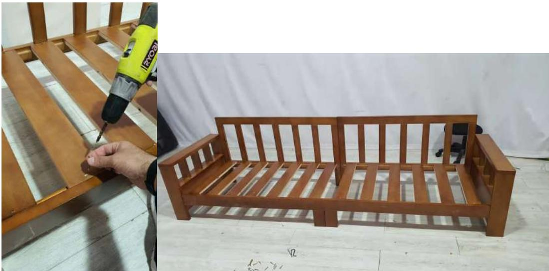
Drill the screws on the frame slats to make the base. Try to leave equal amount of space between each part.
