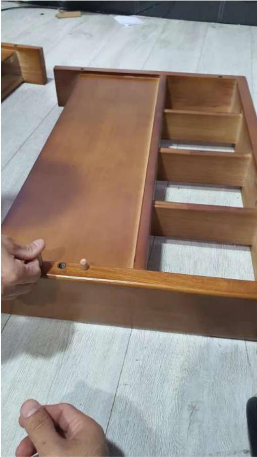
Put the wooden bars and round long thread screw in the both side arms of the sofa as shown in pic
